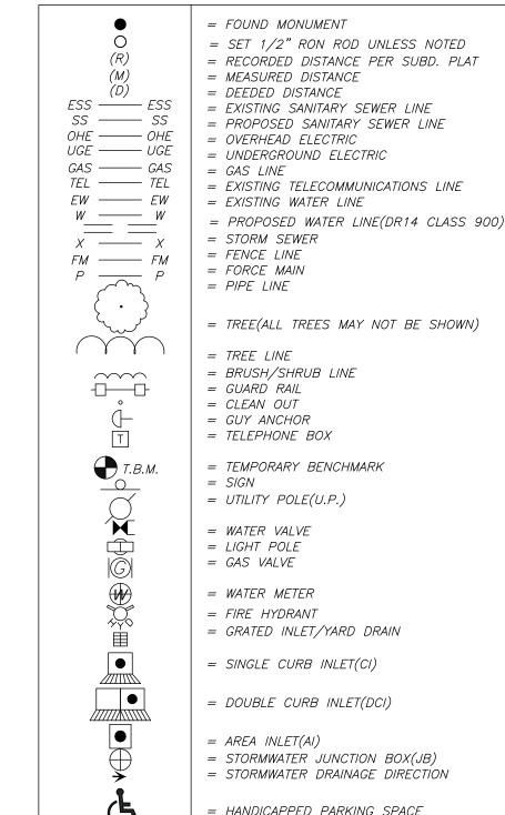
= SINGLE CURB INLET(CI) = DOUBLE CURB INLET(DCI) = AREA INLET(AI) = STORMWATER JUNCTION BOX(JB) = STORMWATER DRAINAGE DIRECTION = HANDICAPPED PARKING SPACE = FINISHED GRADE SPOT ELEVATION = TOP BACK OF CURB = FLOW LINE = TRAFFIC FLOW DIRECTION = WATER LATERAL = SANITARY LATERAL = EXISTING SANITARY MANHOLE(MH) = PROPOSED SANITARY MANHOLE(MH) = STREET LIGHT = EXISTING ASPHALT PAVEMENT = PROPOSED ASPHALT PAVEMENT = EXISTING CONCRETE Δ ..... A V . . A 4. = PROPOSED CONCRETE
